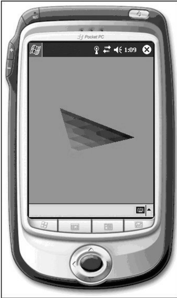
Fig. 5.1. In the rendered triangle the color of each vertex is blended smoothly across triangle surface. We have set Color0.ToArgb() as red, Color1.ToArgb() as green, and Color1.ToArgb() as blue.
